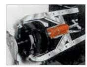
Flexible coupler is removed from electric motor shaft with 2-jaw puller.
