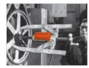
2-jaw puller reaches through spokes of gear to grip hub. Hand pump supplies hydraulic power.
