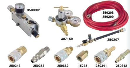
No. 307159 - Pressure reducing valve. Allows use of bottled gases to operate jacks Includes No. 250341 female and No. (works on CGA-580 Nitrogen/Argon/Helium bottles). Contains standard bottle fitting on inlet and 1/4" industrial interchange (female) outlet. Wt., 1.8 kg
