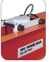
Cylinder is easily moved across width of upper bolster.
