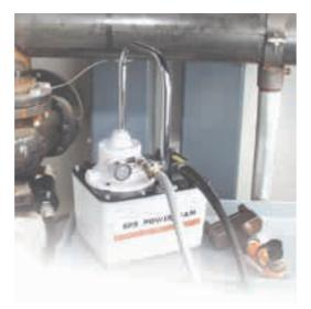
The PA17 used with a flange spreader
